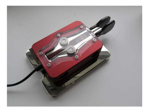
This paddle is intended to be used /P or /A as well as in the shack. The totally enclosed, lightweight, mechanism can be used on its own (when /A or /P), or fixed to a heavy base (for home use) by magnets that hold on to the bolt heads inside the rubber feet.
