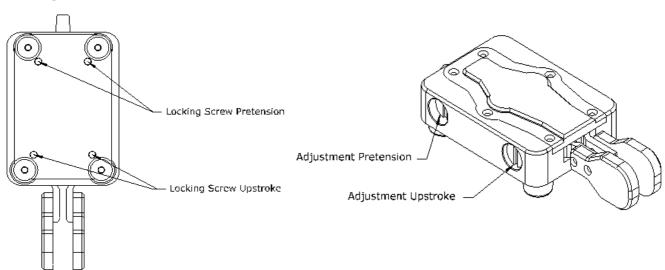
To ensure safe fit of the lever in the optional magnet base 206119 the slotted cylinder screws in the rubber foots can be adjusted to the magnets of the magnet base by screwing them in or out minimally. The key needs to be firmly attached to the magnet base to ensure safe and reproducible operation.
